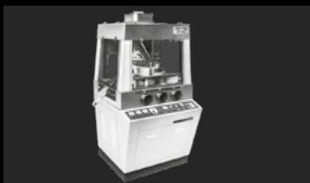
**1970** Fette Compacting develops the P 2000 and P 3000 models, marking the beginning of the era of high-speed tableting presses. For the first time, these machines enabled the production of large batches with exact dosing.
