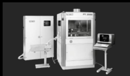
**1982** At Achema 1982, Fette Compacting presents the PT 2080, the world's first computer-controlled tableting press. For the first time, it is possible to control the press and its peripherals via a uniform terminal and to log all process data.
